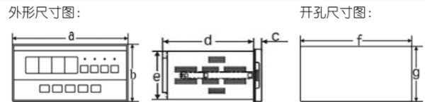
Table with 8 columns: 规格, a (mm), b (mm), c (mm), d (mm), e (mm), f (mm), g (mm). Rows include 160x80, 96x96, 96x48, and 72x72 models.
